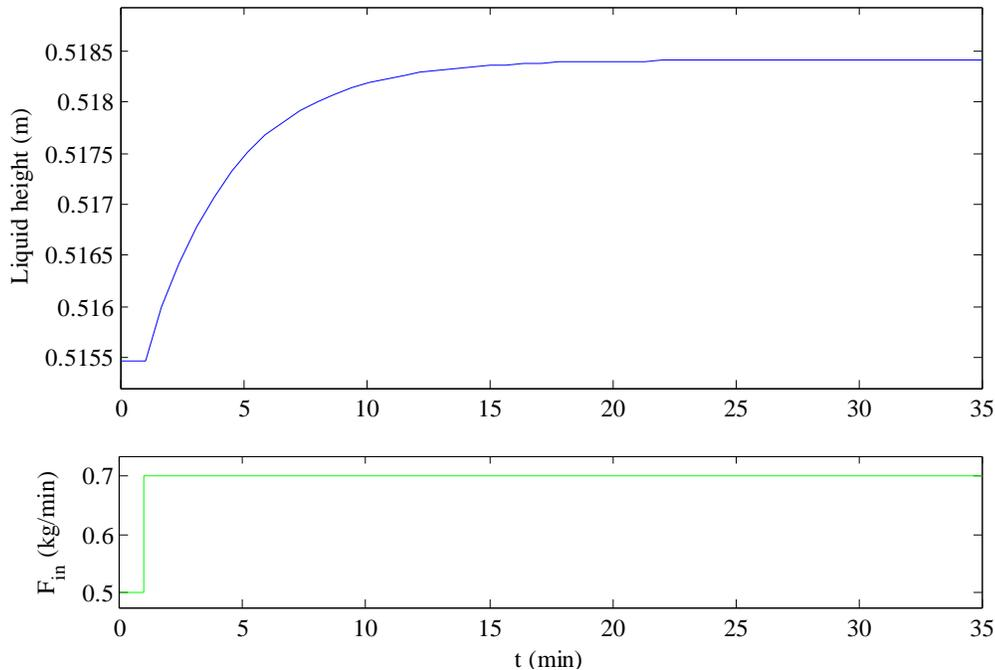
**Figure 5. Dynamic response of liquid height to a +0.2 kg/min step change in feed flow rate**
