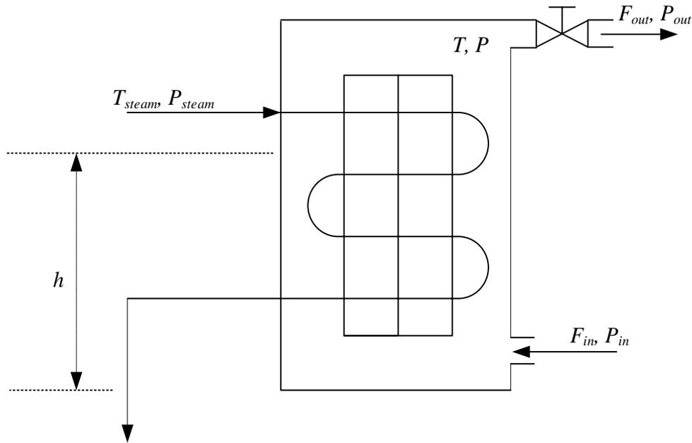
Figure 1. A schematic diagram of an evaporator
