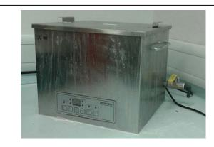
Fig. 3. Ultrawave Precision Ultrasonic Cleaning Machine
