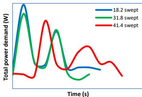
**Figure 9.** Total energy demand milling a toolpath at  $f_z$  0.55 *mm/tooth*
