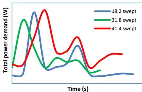
**Figure 8.** Total energy demand milling a toolpath at  $f_z$  0.19 *mm/tooth*
