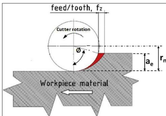
**Figure 1.** Cutter engagement with workpiece adapted from [14]
