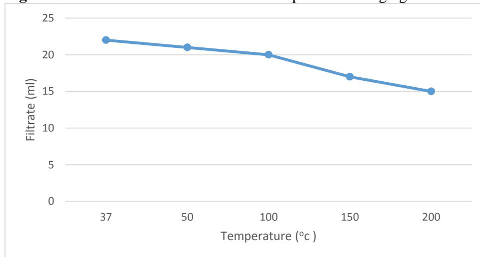
The effect of aging was also studied on the fluid loss test. A good mud must keep the loss of fluid to the formation as minimal as possible while preventing excessively thick filter cake. Thinner and less permeable are thus the desired characteristics of a good filter cake. It was observed that the filtrate decreased with an increase in aging time (figure 5).
