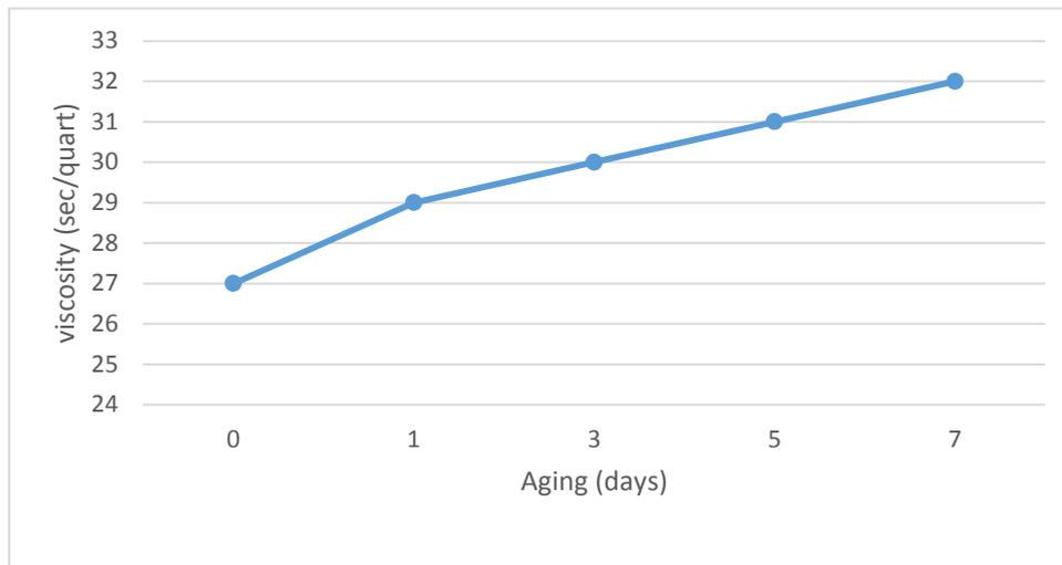
**Figure 9:** Viscosity as a function of aging
