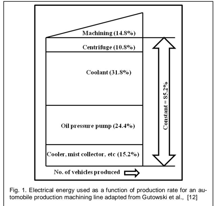
Fig. 1. Electrical energy used as a function of production rate for an automobile production machining line adapted from Gutowski et al., [12]
