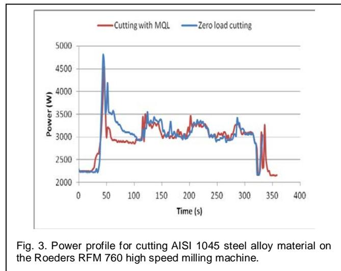
Fig. 3. Power profile for cutting AISI 1045 steel alloy material on the Roeders RFM 760 high speed milling machine.
