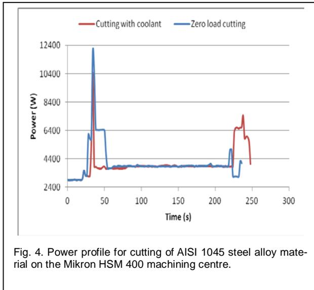
Fig. 4. Power profile for cutting of AISI 1045 steel alloy material on the Mikron HSM 400 machining centre.
