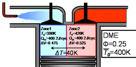
Fig. 3. Calculation condition (DME, Thermal stratification, 2-zones)
