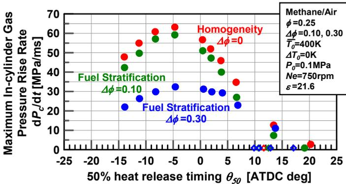
Fig. 16. 50% heat release timing and maximum in-cylinder gas pressure rise rate (Methane, Fuel stratification, 5-zone)
