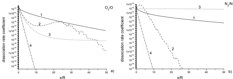
Fig. 4. Averaged dissociation rate coefficient  $k_{diss}^{(mol)}$  ( $\text{m}^3/\text{s}$ ) versus  $x/R$  in a conic nozzle. (a)  $\text{O}_2/\text{O}$ ,  $T_* = 4000 \text{ K}$ ,  $p_* = 1 \text{ atm}$ ; (b)  $\text{N}_2/\text{N}$ ,  $T_* = 7000 \text{ K}$ ,  $p_* = 1 \text{ atm}$ . Curves 1: state-to-state model; 2: two-temperature anharmonic oscillator model; 3: two-temperature harmonic oscillator model; 4: one-temperature model.
