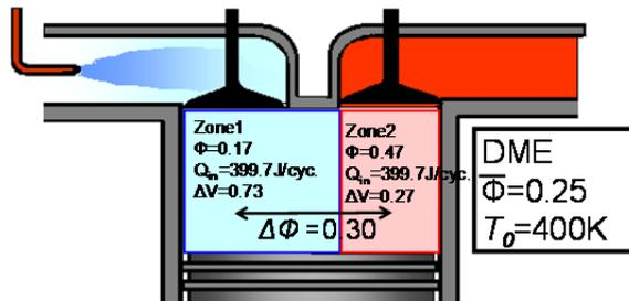
Fig. 8. Calculation condition (DME, Fuel stratification, 2-zones)
