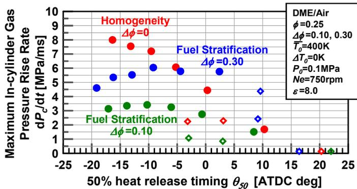
Fig. 14. 50% heat release timing and maximum in-cylinder gas pressure rise rate (DME, Fuel stratification, 5-zone)
