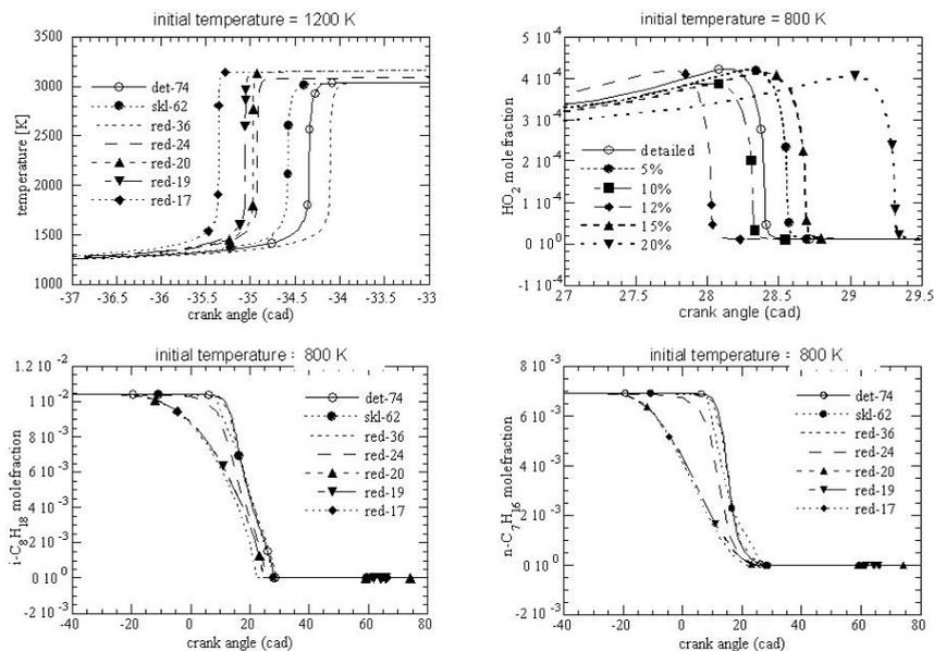
Fig. 9. Calculated temperatures and mole fraction profiles for the end-gas of an SI-engine. Top left: temperature profile, top right:  $\text{HO}_2$  mole fraction representing a radical profile, bottom: fuel profiles, the iso-octane and the n-heptane. Different reduced mechanisms are compared with the detailed and skeletal mechanisms (Soyhan et al., 2000)
