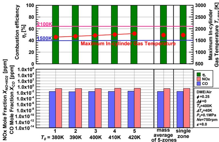
Fig. 17. CO and  $\text{NO}_x$  mole fraction in exhaust gas, combustion efficiency and maximum in-cylinder gas temperature (DME, Thermal stratification, 5-zones)
