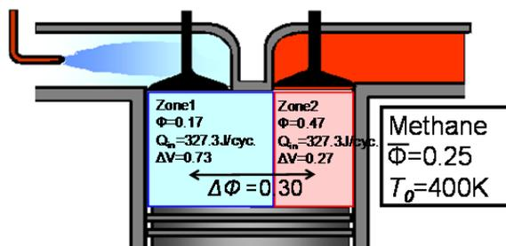
Fig. 9. Calculation condition (Methane, Fuel stratification, 2-zones)
