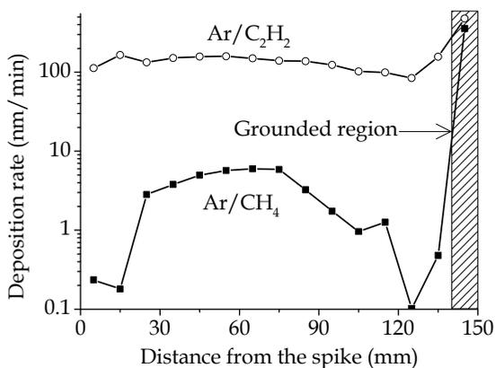
Fig. 8. Deposition rate of carbon based film inside of quartz tube by filamentary discharge in Ar/C<sub>2</sub>H<sub>2</sub> and Ar/CH<sub>4</sub> mixtures.
