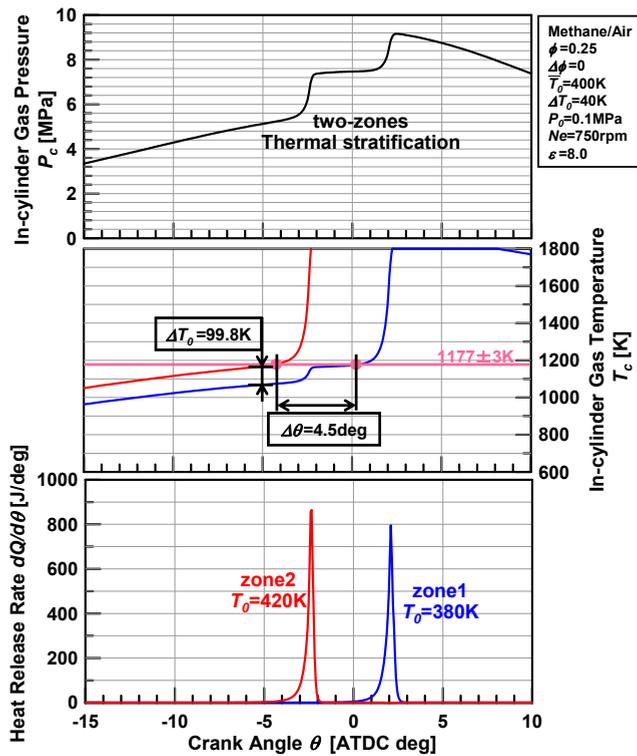
Fig. 7. Histories of in-cylinder gas pressure, in-cylinder gas temperature and heat release rate (Methane, Thermal stratification, 2-zones)
