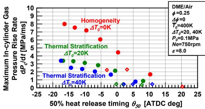
Fig. 13. 50% heat release timing and maximum in-cylinder gas pressure rise rate (DME, Thermal stratification, 5-zone)
