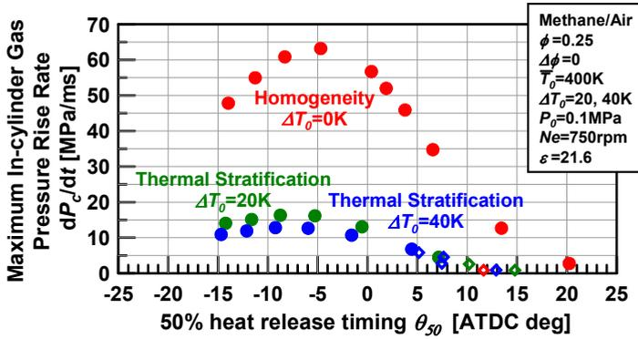
Fig. 15. 50% heat release timing and maximum in-cylinder gas pressure rise rate (Methane, Thermal stratification, 5-zone)
