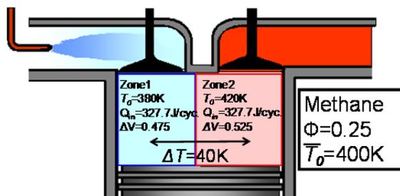
Fig. 4. Calculation condition (Methane, Thermal stratification, 2-zones)
