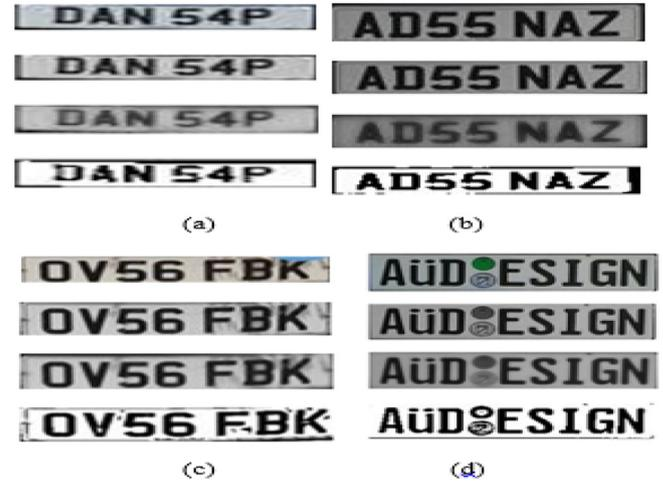
**Fig. 7.** GrabCut, gray-scale, noise removal and binarization of localized plates of vehicle images (a), (b), (c) and (d).
