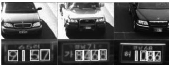
Fig. 1. Blob detection using Dynamic Programming-Based Method (Kang, 2009).
